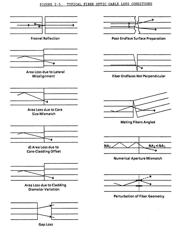
Chap 2 Par 26 (c) <u>Gap Loss</u>. A gap between the fibers results in some of the light rays emanating from the transmitting fiber diverging beyond the cone of the receiving fiber.
