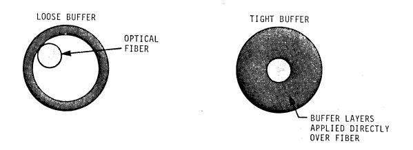
(1) <u>Loose Buffer</u>. In loose buffer construction, the fiber is contained in a plastic tube that has an inner diameter considerably larger than the fiber itself. The loose tube isolates the fiber from the exterior mechanical forces acting on the cable. By controlling the amount of fiber inside the tube, the amount of allowable temperature variation can be increased and, therefore, the degree of attenuation over a temperature range is minimized.
