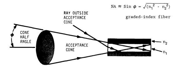
$n_1 = maximum$  refraction index of core  $n_2 = index$  of refraction of cladding
