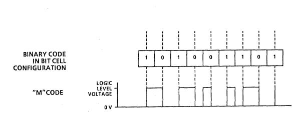
FIGURE 3-4. MANCHESTER "M" ENCODING SCHEME
