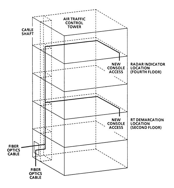
SECOND FLOOR RUN 95 FEET FROM ENTRY FOURTH FLOOR RUN 125 FEET FROM ENTRY
