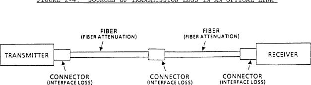
FIGURE 2-4. SOURCES OF TRANSMISSION LOSS IN AN OPTICAL LINK
